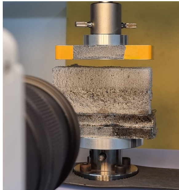
Figure 2: Experimental setup of the compression experiments. The samples are sprayed with black ink to increase the contrast for the high speed video recording.
