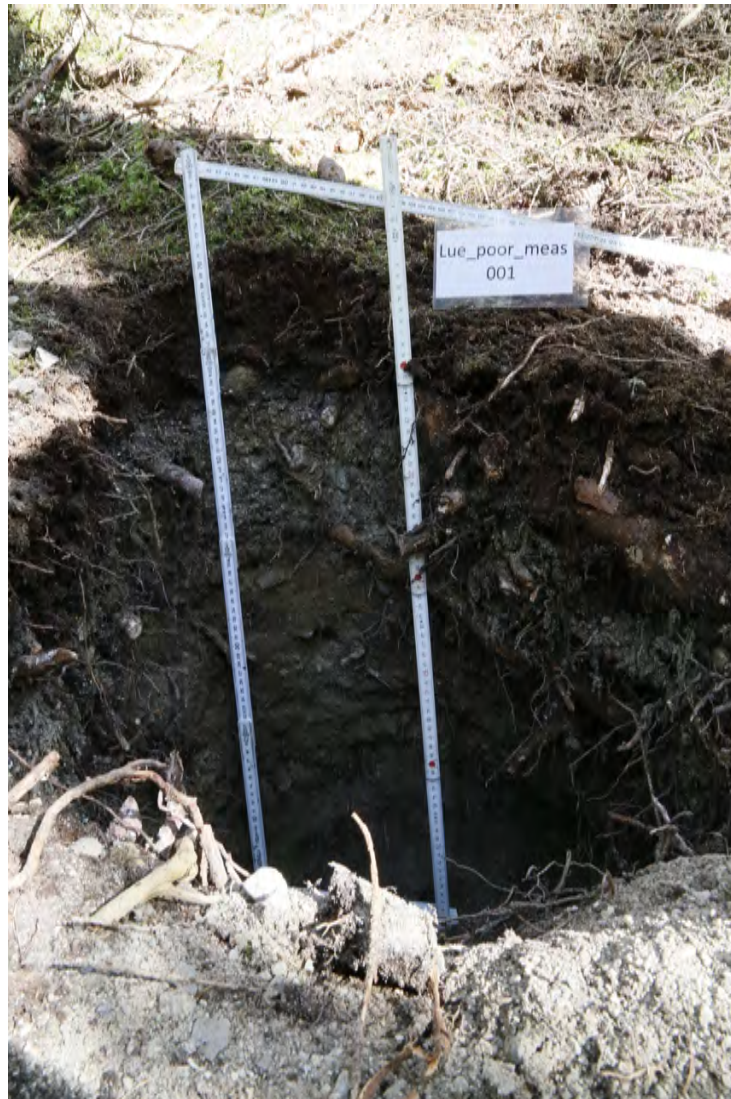
Figure 54: Soil profile at Poor_meas001 with depth of 60 cm. The soil profile was done during the installation of the sensor and data loggers.
